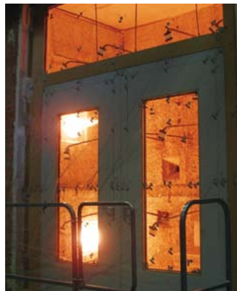
T90 fire test
